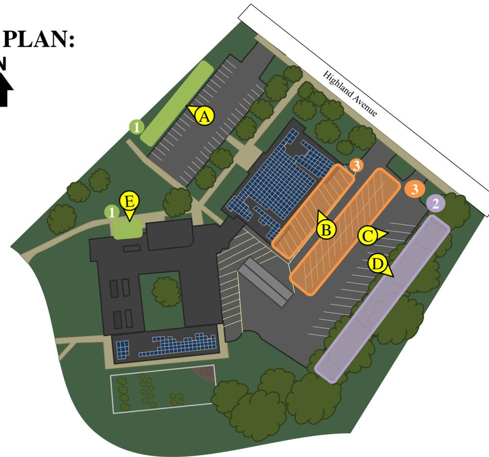
**1 BIORETENTION SYSTEMS:** Curb cuts along the western edge of the western parking lot can feed runoff from the lot to a bioretention system or rain garden where it can be treated and allowed to infiltrate. Another rain garden along the edge of the school can be used to capture runoff from a portion of the building's roof. The gardens can also provide habitat for birds, butterflies, and pollinators.
